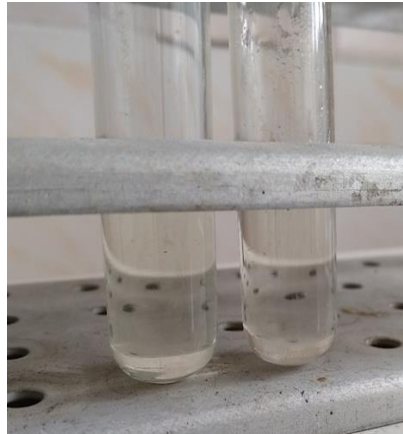
Fig. 13. The growth M. bovis on the Sauton medium: left test tube – GKP-305 (50 µg/mL, no growth), right test tube – control (growth in the form of intense flakes and plaits)
