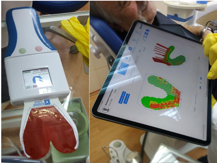
Fig. 1. Methods of digital registration of occlusal pressure distribution OccluSense by Bausch.
