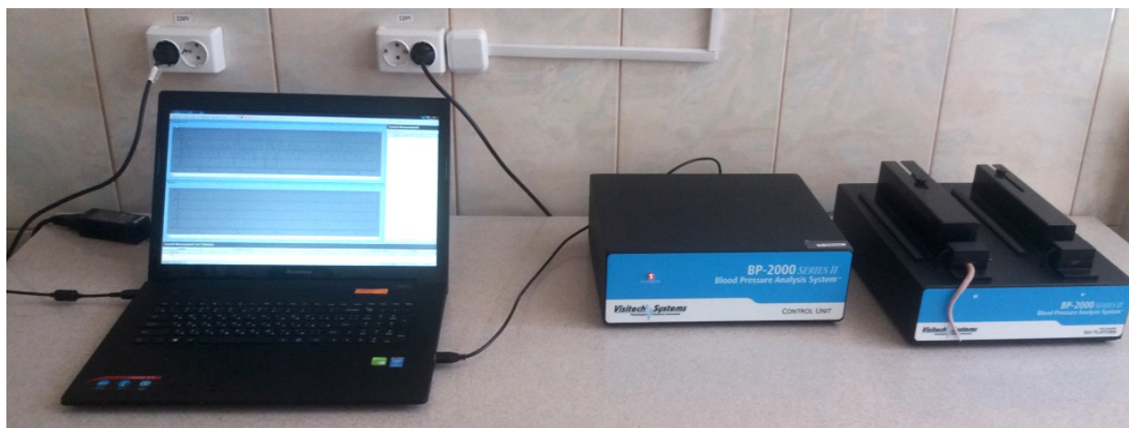
Fig.1. Definition of blood pressure using the system of non-invasive blood pressure measurement Blood Pressure Analysis Systems TM BP-2000 Series II.
