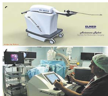
Fig. 31. Hardware complex for performing robot-assisted flexible urethroscopy "Avicenna Roboflex "(ELMED, Ankara, Turkey) (a), control console-B)
