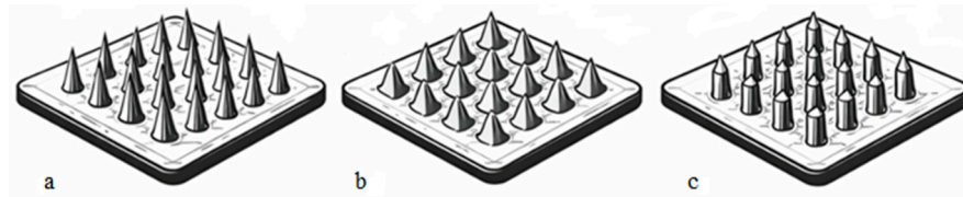
Figure 2. Shapes of microneedle systems ((a) conical; (b) pyramidal; and (c) cylindrical).
