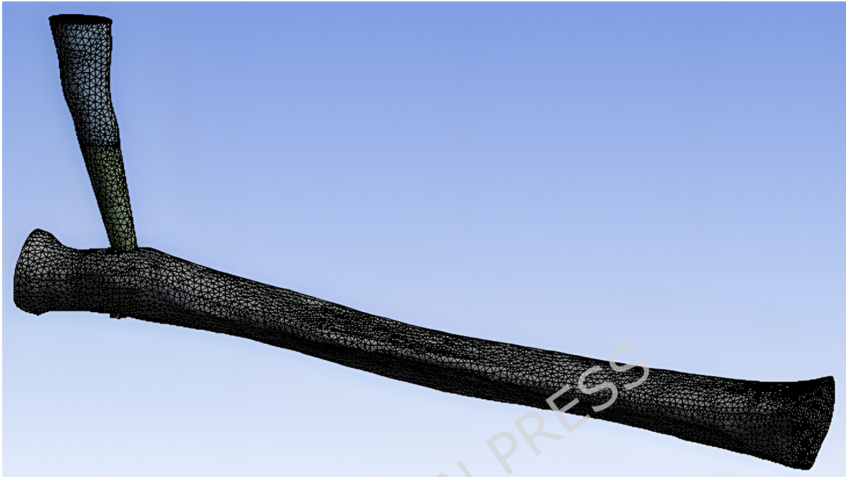
Fig. 8 Finite element mesh of the models. Tetrahedral mesh with maximum element size of 1 mm applied to all components (radius, tendon, fixation system, and button).
